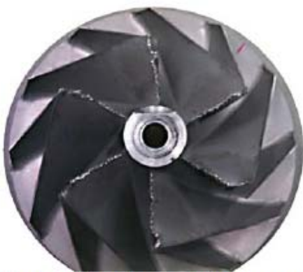
Foreign object damage to the compressor wheel.
